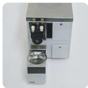
FlexyCUBE operating with one each pump and balance, allowing gravimetric dosage
