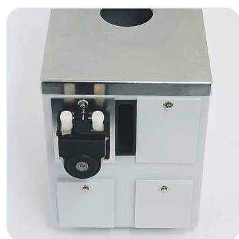
FlexyCUBE operating with a single peristaltic pump, used for volumetric dosage
