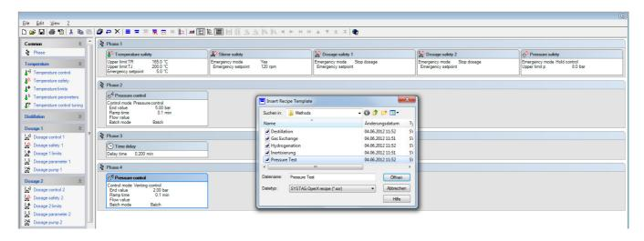
Recipes are set by simply dragging and dropping the individual operations into defined recipe phases. Critical sequences such as inerting or leak tests can be combined into pre-defined methods, thus making them available to every user for his/her recipes.
