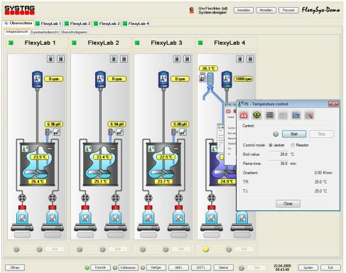
vated by a simple click on its symbol to open a subwindow with further parameters. Data logging & trending is possible at any time during the process.
