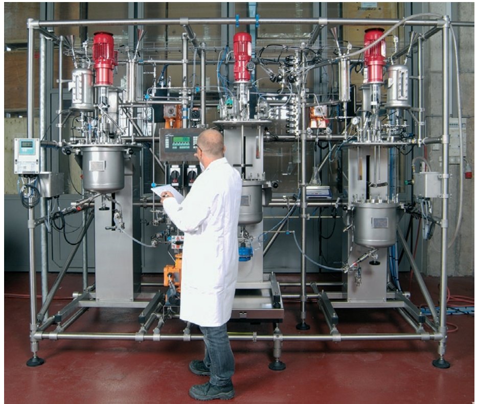
Fig. 2: The automated turn-key pilot plant for suspension-polymerisation was automated based on FlexyConcept.
