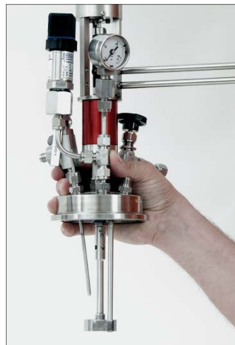
Illustration 3 View of temperature sensor (oblique), inlet/sampling tube and stirrer
