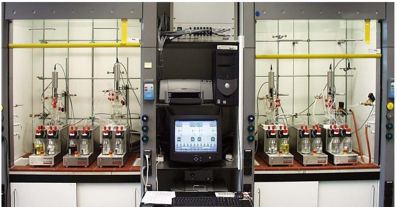
4-units FlexyLab with additional 3rd dosage for each reactor
