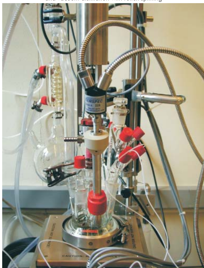
Reactor with mid-IR Fibre Optics, multiple dosages and vacuum distillation with reflux splitting
