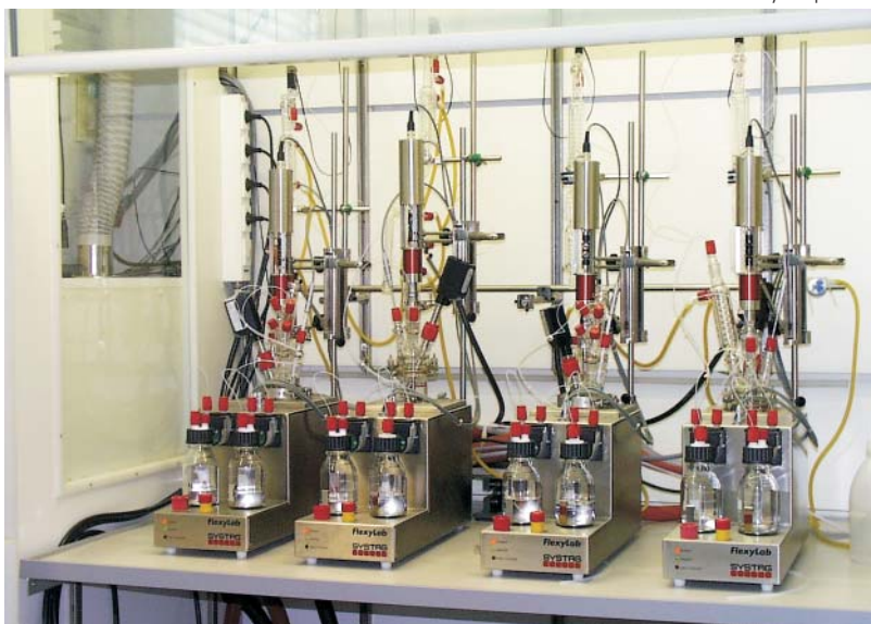
4-units FlexyLab Fast Track with 100 ml reactors and 4 Lasentec Particle Size Analyzer probes
